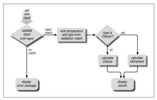
Figure 2-2: Temperature-conversion program's logic flow
